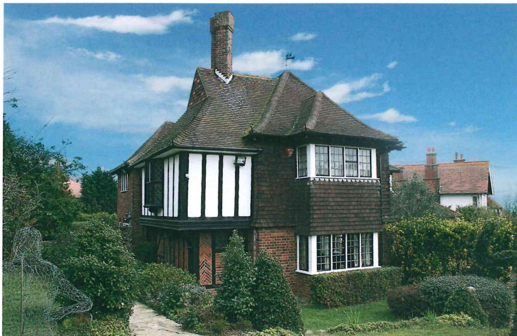
Figure 2. Poynings, on the North Foreland Estate to the north of Broadstairs, designed for William Morris in 1924. The half-timbered first-floor bathroom, left, was added four years later (Timothy Brittain-Catlin)
