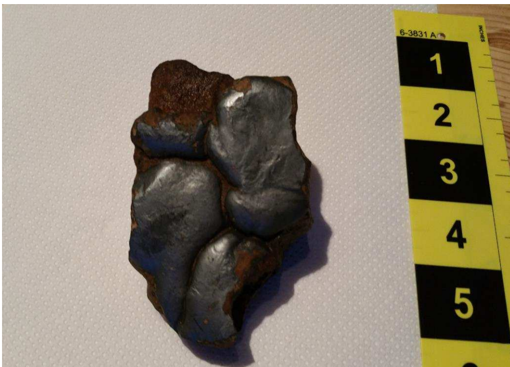
Figure 58: Tap slag found by the author walkover surveying the Gallant's Lane possible iron working site, the first such if proved of Roman provenance outside of the Weald in Kent. Simon Elliott.
