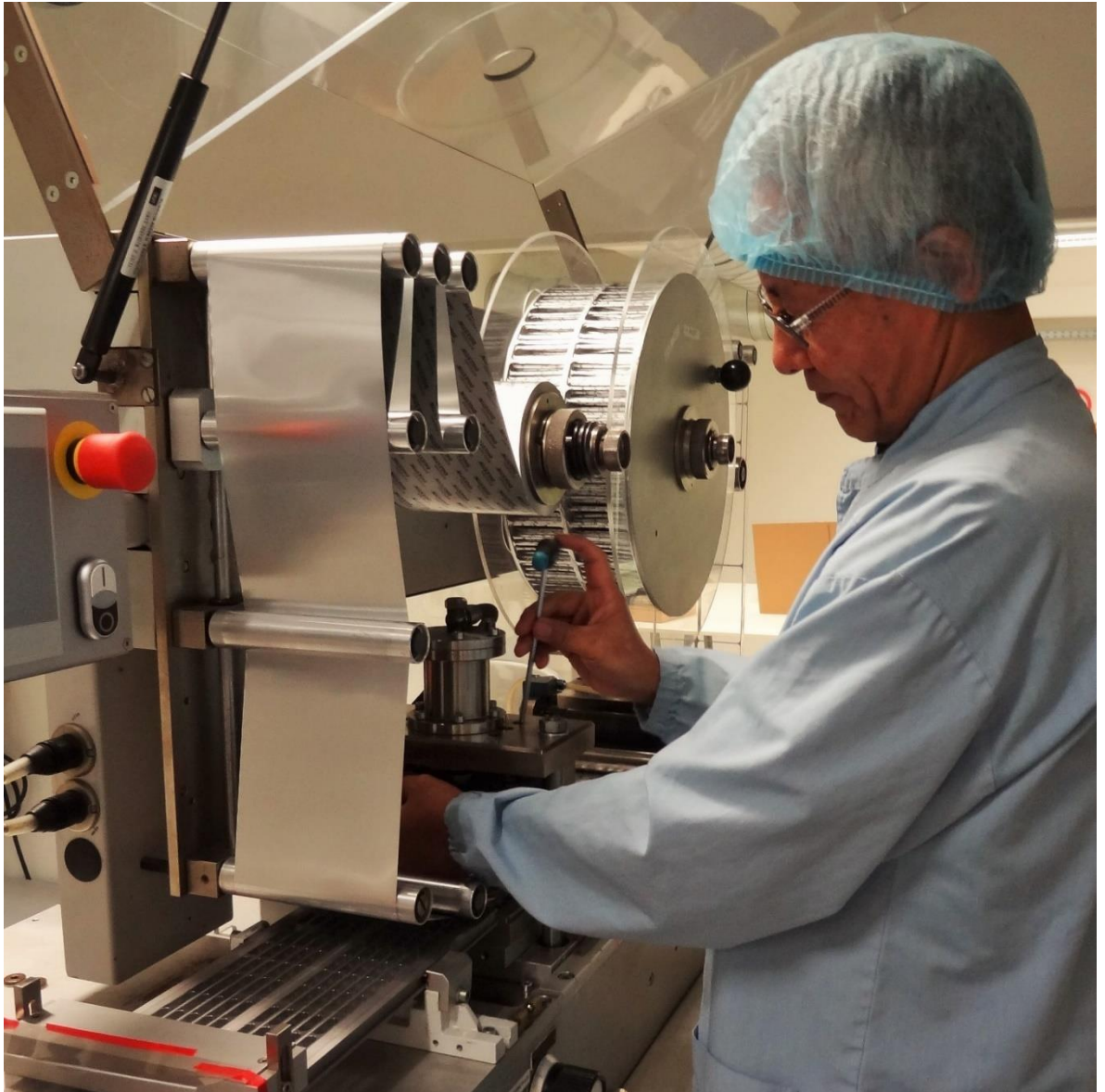
Figure 3.3. Pema manually tweaked the position of the sealing compartment, which applies heat and pressure to cover and seal the filled plastic pockets with aluminium foil. In subsequent steps, the batch number and expiry date is impressed, the blister packs (containing twenty capsules each) are cut out, and then slide down steadily towards the packaging workers. His intervention was called for in this instance because two blister pockets were not being perfectly separated from each other in a small minority of blisters.
