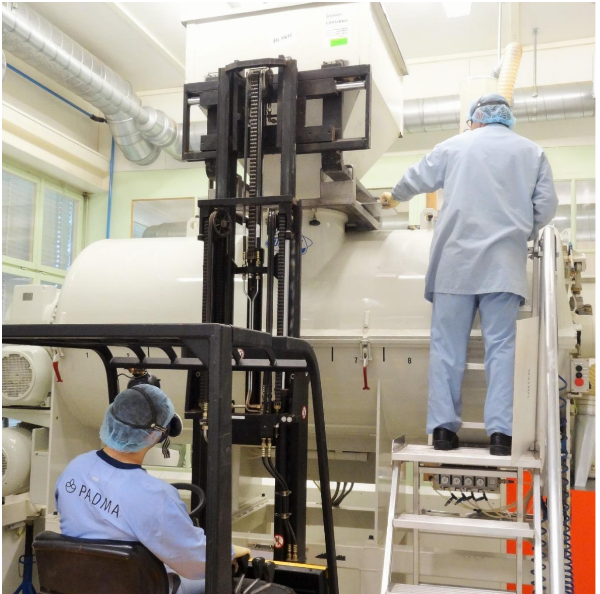
Figure 3.1. Mevlan watched from the forklift truck as Liman opened the shaft of the dosing container to release the powdered mixture into the mixing machine. A proportion of the material in the form of hard chunks (of powdered Phyllanthus emblica fruits) was temporarily blocked by a grid covering the mixer.
