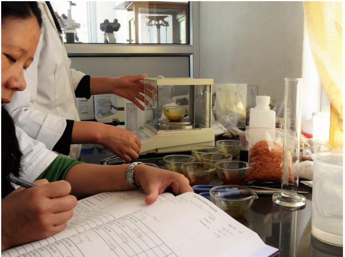
Figure 4.3. The final step in the determination of the alcohol extractive value of gurgum (here identified as Carthamus tinctorius L.). Norlha is weighing the dish with the dried extract, and Phurpu writes down the result and then calculates the percentage (photograph taken on 23 April 2014).
