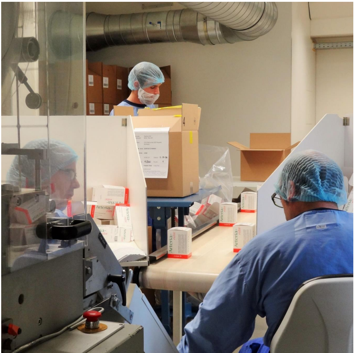
Figure 3.4. Manual packaging of Arteria-vita, a product of the PADMA 28 family (with identical ingredients to both Swiss PADMA 28 and PADMED Circosan) that is marketed specifically to Swiss doctors by the independent company Permamed AG. The blisters were taken from the blistering machine (left) and put into the boxes together with the package leaflet by hand before the new packaging line was installed in early 2015.
