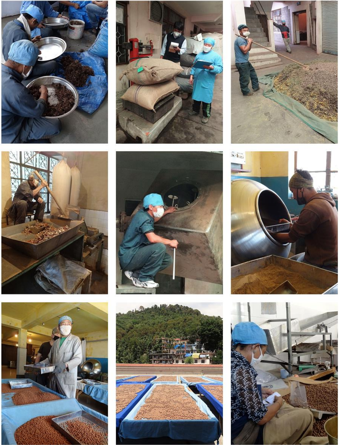
Figure 5.6. The main steps of rilbu production at Men-Tsee-Khang, left to right and top to bottom. Pre-processing (manual sorting of pangpö ), weighing and compounding of raw materials (in this case Tikta-8 ), grinding, mixing, pill rolling, size checking, drying ( Agar-35 ), and counting, labelling and packaging. Photographs taken by the author, Spring 2014. Courtesy Men-Tsee-Khang.
