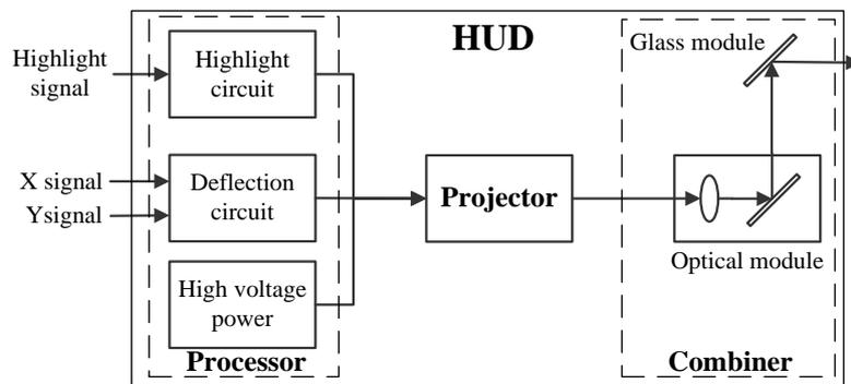
Fig. 3. The structure of HUD system [33].
