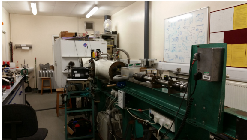
Figure 3.1: Image of the University of Kent's Two-Stage Light Gas Gun as used for majority of the work in this thesis.
