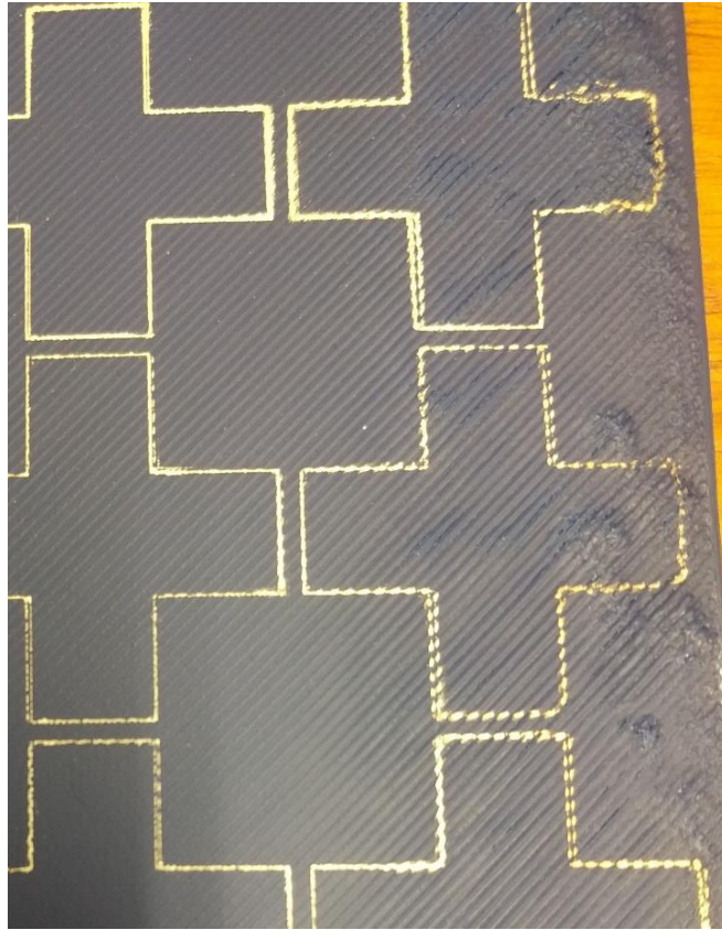
Figure 5-14 Silver ink depositing issue on the corners of the element
