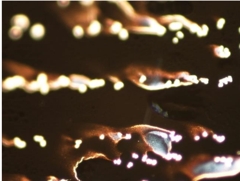
Figure 8-13 Zoomed in photo of the pockets on the surface of the printed material
