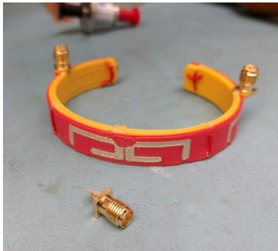
Figure 7-11 Printed bracelet with a broken off SMA connector
