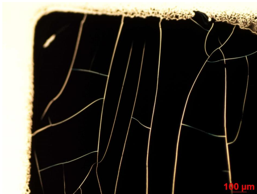
Figure 8-14 Overview of the level of cracks on the surface of the printed material
