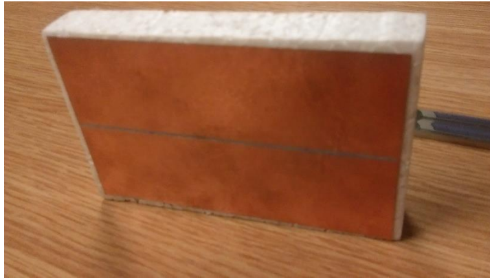
Fig. 9c Slot antenna with anSMA connector
