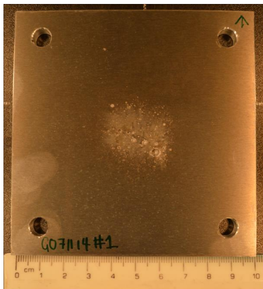
Figure J11 Target plate for natural gypsum projectile, shot I.D. G071114#1 ( 5.86 \text{ km s}^{-1} ).
