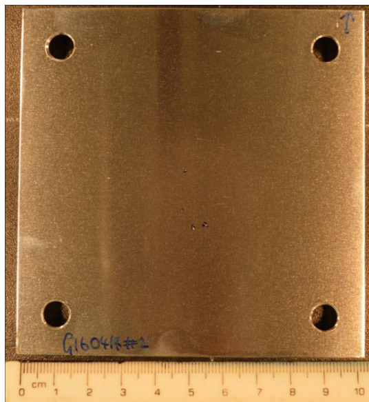
Figure J3 Target plate for hydrous PoP powder projectile, shot I.D. G160414#2 ( 4.38 \text{ km s}^{-1} ).
