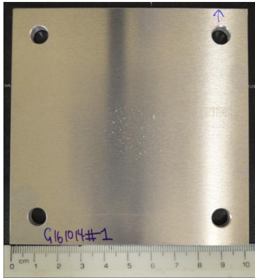
Figure J7 Target plate for natural gypsum projectile, shot I.D. G161014#1 ( 3.97 \text{ km s}^{-1} ).
