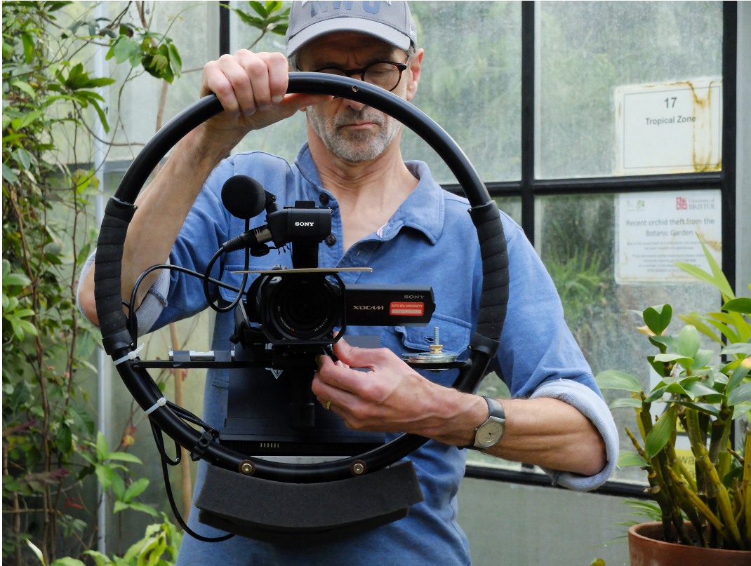
Figure. 63. The Glasshouse (Lewis-Smith 2016). Sony PXW x70 camera housed in 'Fig-Rig'.
