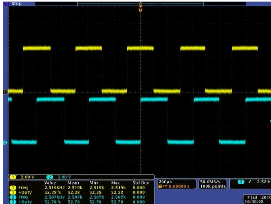
Figure 4.6: Output signals of the encoder assembled on the motor shaft
