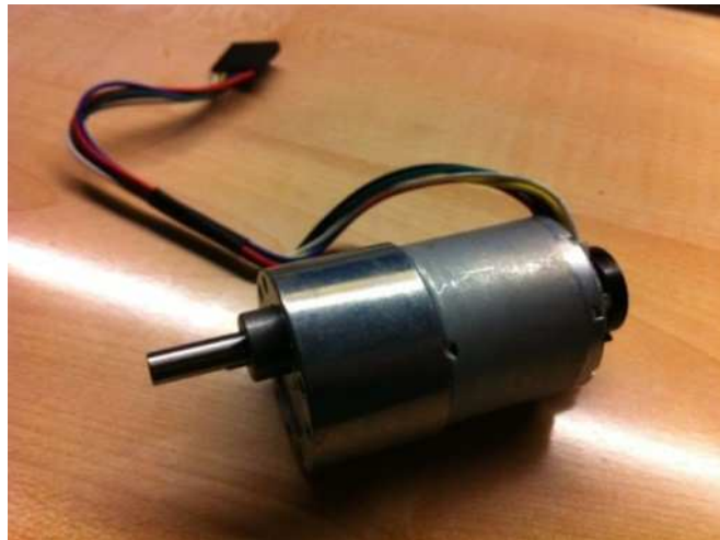
Figure 4.5: Pololu 12v 50:1 Gear Motor w/Encoder
