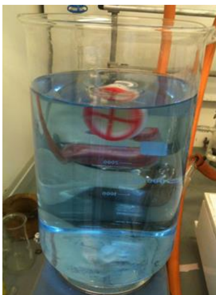
Figure 4.14 : PMDETA/water dialysis tank after 48 hours. The polymer sample was dissolved in water within the holder, behind dialysis tubing. The blue colouration is due to the presence of chelated copper ions.
