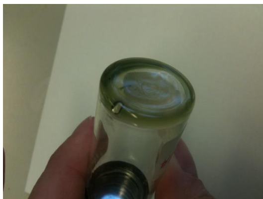
Figure 4.13 : A portion of sample P1, showing the green colour of the polymer that persisted following passage through alumina columns and precipitation into hexane.
