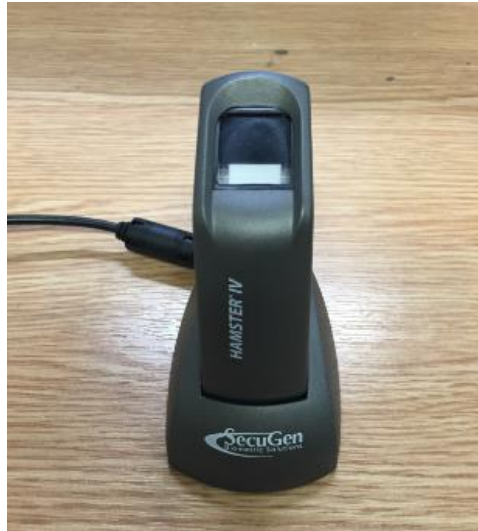
Figure 2.6: The optical fingerprint sensor (SecuGen Hamster IV).
