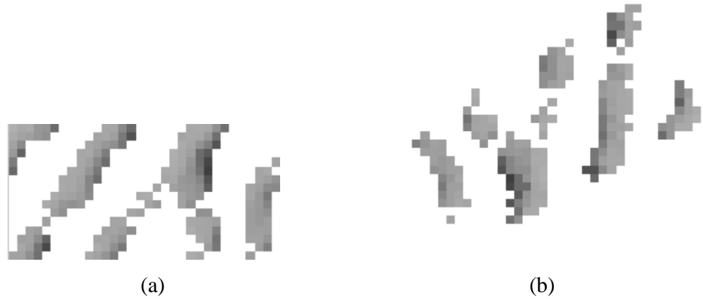
Figure 3.13: (a) The block of the pre-processed image O(i, j) ; (b) the block image O_2(i, j) , which is rotated from Figure 3.13 (a) by the average of angle degrees so as to bring it into vertical alignment.
