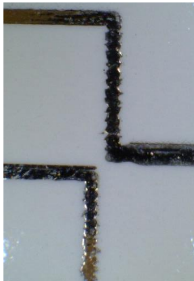
(b) Elements microscopic photos ( w = 0.2 mm)
