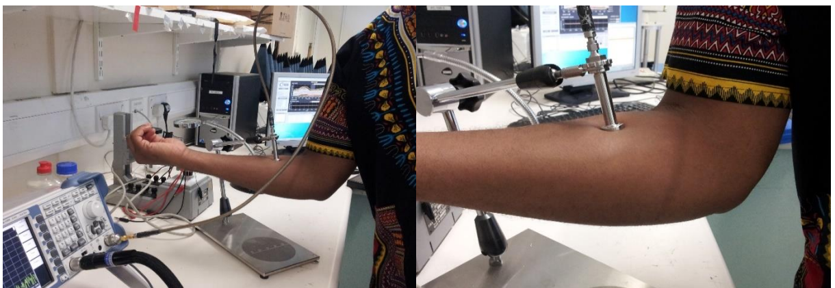
Fig. 3.17 Measurement of Skin Dielectric Parameters with the DAK
