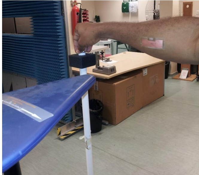
Fig. 3.16 Transfer Tattoo Tag performance measurement setup
