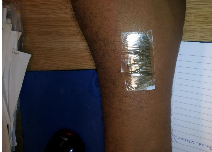
Fig. 5.22 Crease on the Inkjet Printed Transfer Tattoo Tag During Use
