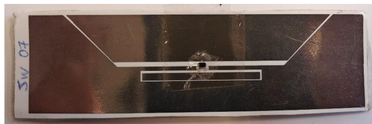
Fig. 6.10 Inkjet printed Tag using conductive ink
