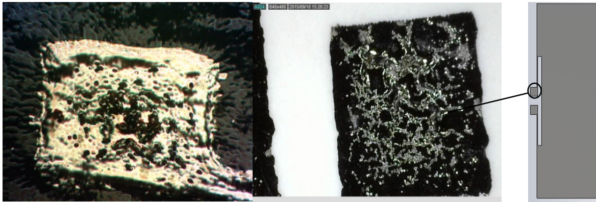
Fig. 5.6 Pinhole defects on the RFID tag port
