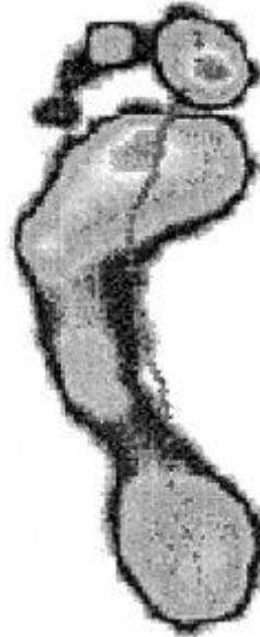
Figure 1. Example of footscan image, showing maximal pressures under a left human foot during ground contact in a bipedal walking sequence. Dotted line in foot illustrates displacement of center of pressure (dot interspace, 4 msec).
