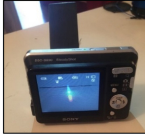
Fig. 8. Image of 10.1 MP camera attached to the spectrograph. The diffracted light entering the slit can be captured.
