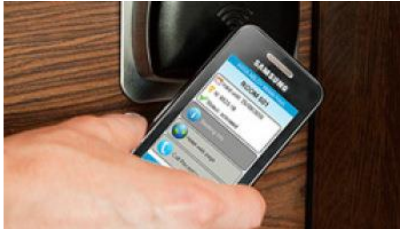
Figure 2.35 NFC enabled phone being used as a key at Clarion Hotel, Stockholm
