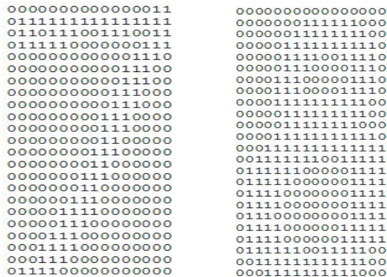
Figure 3.2(b): A binarised handwritten digits from a benchmark database known as CEDAR.
