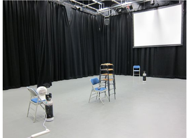
Fig 7: Releasing CO 2 as a tracer gas in the studio.
