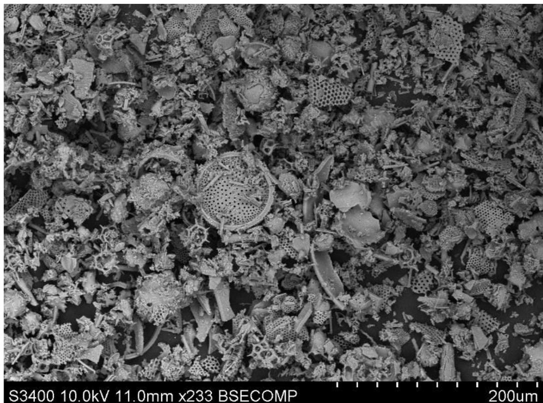
Figure 36: This image also seen in chapter 2 shows an SEM image of a field of diatomaceous fossils sourced from the un-shot control. Here the diatoms were frozen within a sabot and then included in the water bag target. This was then filtered and imaged. This particular image was produced using the back scatter function on the SEM with the magnification set at x233.
