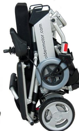
Figure 1.5 Golden Motors lightweight rear-wheel driven transportable PWC (China) Image credit: Golden Motor Technology Co Ltd China
