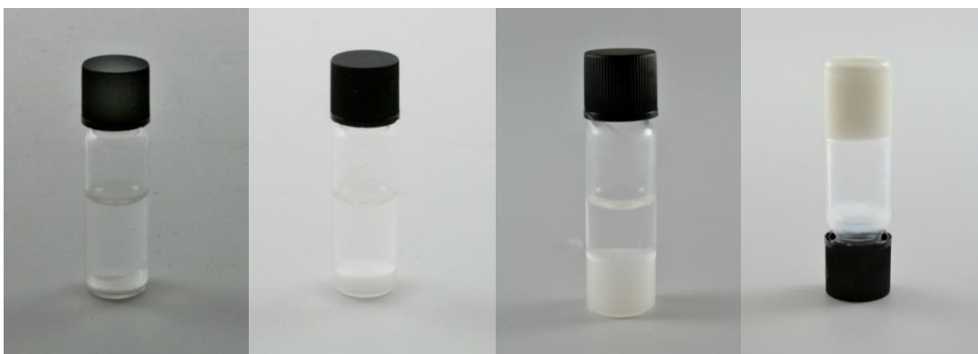
Figure 5.6: Settling and gelating processes observed when dilutions of a dispersion (D1) stabilised by PMMA- b -PODA (S3) were allowed to stand for a period of time; from left to right - 1%, 10%, 20% and 40% solid content.
