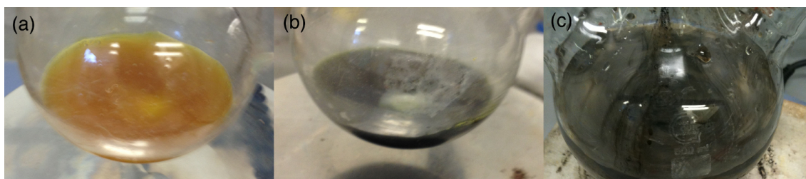
Figure 69: Photos of the co-precipitation/stabilisation reaction of the magnetite/dopamine composite. The starting materials form an orange solution (a), which when exposed to dopamine the solution changes to dark green (b). After addition of ammonium hydroxide a jet black precipitate forms, characteristic of magnetite (c).
