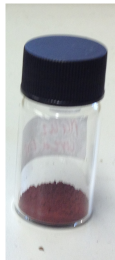
Figure 30: Non-magnetic, red precipitate obtained from the one step urea based co-precipitation reaction.
