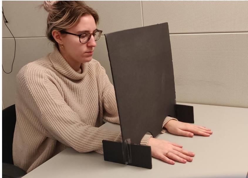
Figure 1: Experimental set-up. The participant sat in a chair with both their hands resting palm-down on a table in front of them. Vision of the hands was obscured using a piece of black cardboard.
