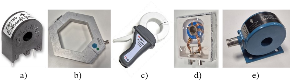
Fig. 5. Evaluated current transformers: a) HFCT1; b) HFCT2; c) HFCT3; d) HFCT4; e) HFCT5
