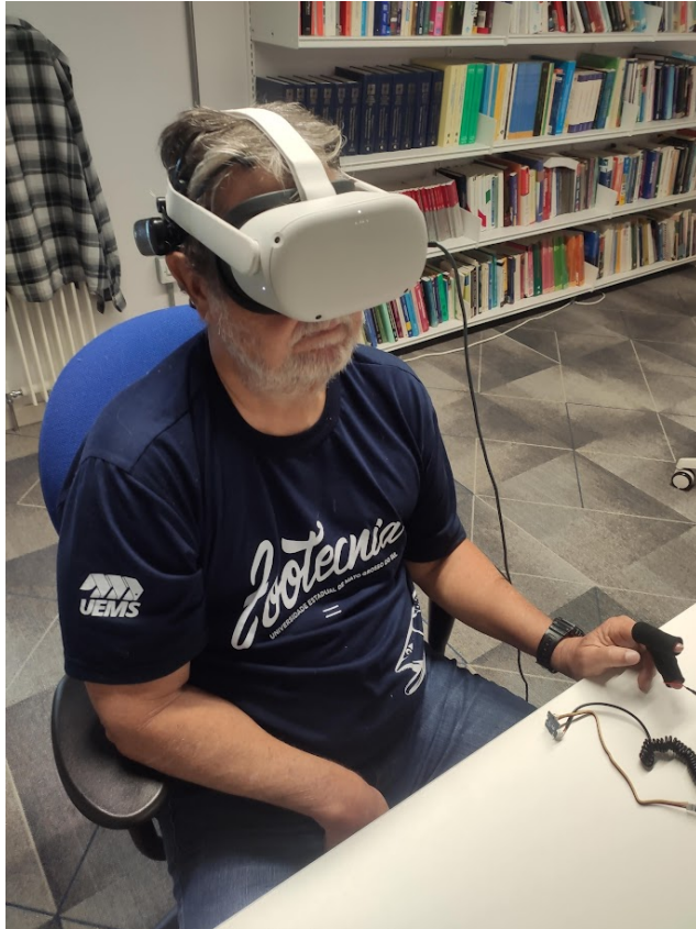
Figure 3: A research participant using the devices for biosignals capture. The Grove GSR attached to the fingers, the EMOTIV EPOC X under the Meta 2. The polar H10 cannot be seeing under the shirt.
