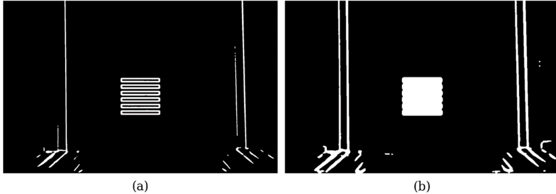
Fig. 16. Binary image containing a marker with a 5.0 mm spatial period at a camera distance of 1.0 m broken into stripe contours (a). Binary image under the same conditions using an image pyramid (b).
