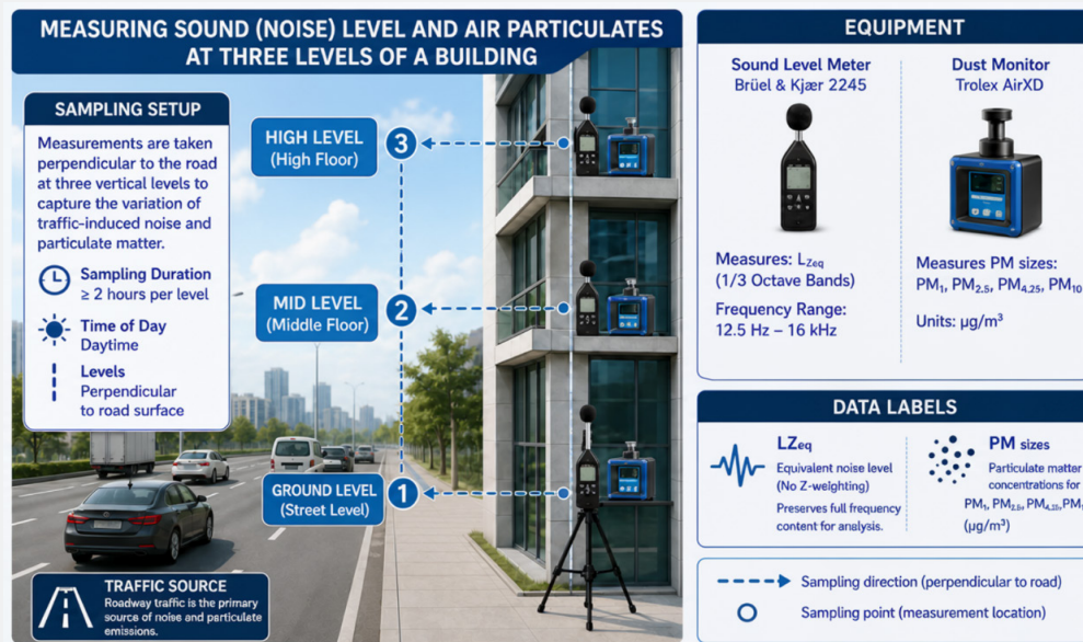
Figure 1: Data collection and sampling setup at three different levels of a building.
