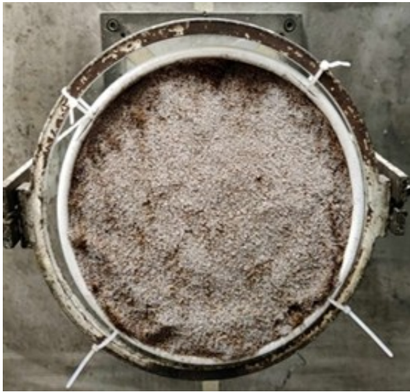
Figure 1: Example pre-impact JSC Mars-1 target mounted to the Kent light-gas gun. The target diameter was 20 cm.
