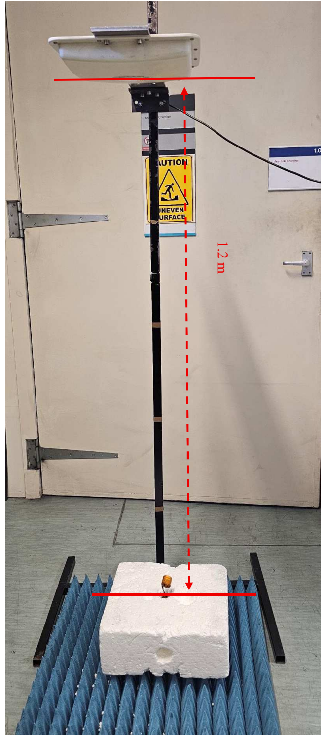
Fig. 5. PPG ring tag 1.2m away from a JadaK ThingMagic M7E RFID reader's antenna.
