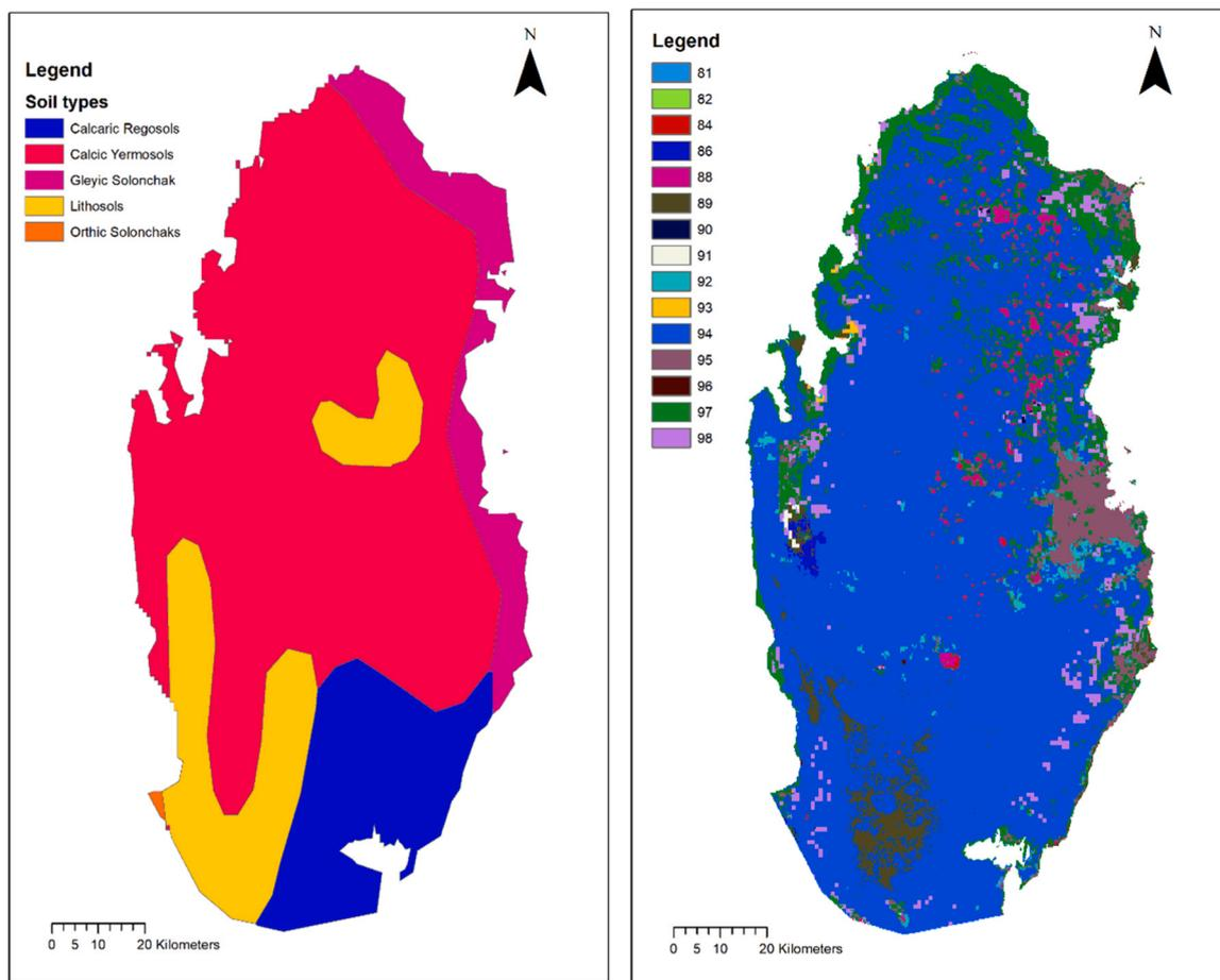
Fig. 9. Soil types and curve number map of the State of Qatar. Source (FAO, 1988).
