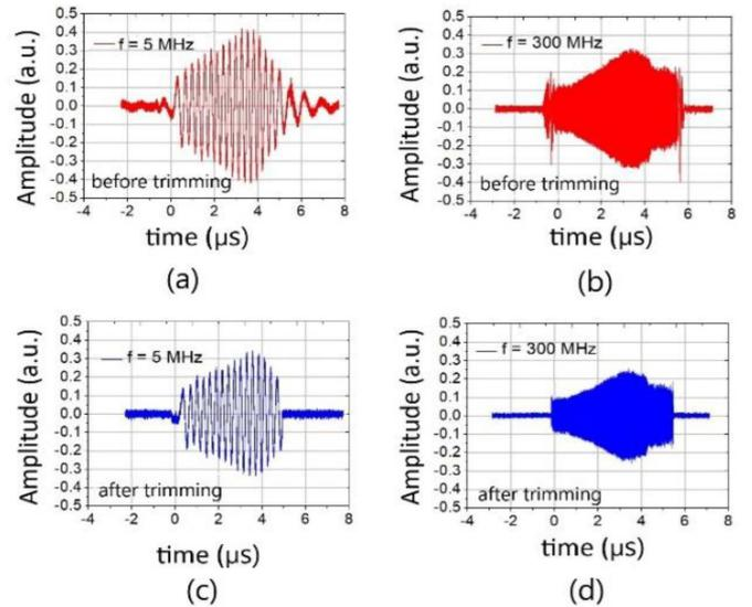
Fig. 2. Two photodetected signals,  $C(k)$ , for two different optical path differences in the Follower interferometer (FI), at input  $i_1$  of the AWG, before being trimmed by the AWG (a) and (b) and after being trimmed by the AWG before storage (c) and (d).
