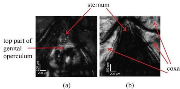
Fig. 11. Two *en-face* OCT images from two different depths simultaneously displayed, using EO regime of operation and masks from the set of 330 obtained via the CLF protocol. (a)  $z = 3.31$  mm ( $f = 142$  MHz); (b)  $z = 4.175$  mm ( $f = 178$  MHz). Image size 2 mm × 2 mm.
