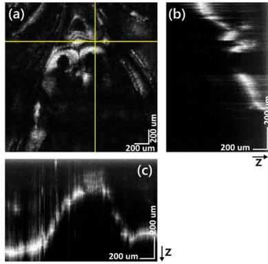
Fig. 10. Orthogonal slicing through the spider, with the depth of the *en-face* image at 3.81 mm (measured in air) (163 MHz) inside the transparent plastic block within which the scorpion is embedded in. Images size: a) 2 mm × 2 mm, b) 1.32 mm in depth measured in air x 2 mm c) 2 mm × 1.32 mm measured in air. All scale bars are 200 μm.
