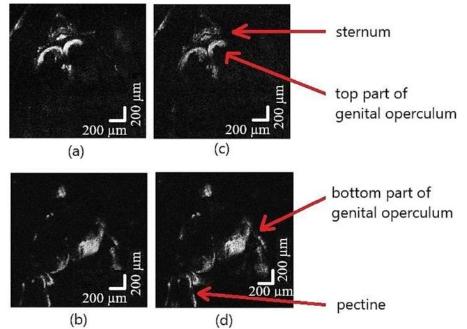
Fig. 12. Comparison of OO regime of operation (a) and (b) versus EO (c) and (d) for two *en-face* OCT images from two different depths at  $f = 70$  MHz (top row images) and  $f = 88$  MHz (bottom row images) [focus was positioned inside the sample at  $\sim 75$  MHz] Image size 2 mm × 2 mm.
