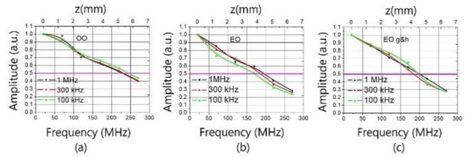
Fig. 5. Decay of sensitivity with OPD for three different scenarios (a) OO, (b) EO, and (c) EO  $g&h$ . All of them were obtained using the  $I&Q$  mixer and LPFs for 1 MHz (black), 300 kHz (red) and 100 kHz (green).
