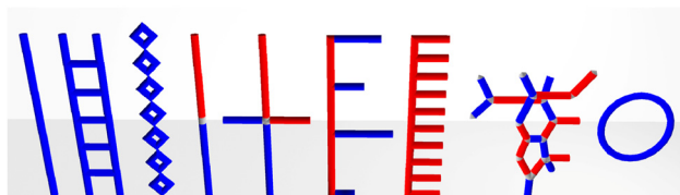
Fig. 1: Classes of macromolecular structures. Left to right: single-strand, ladder, spiro, block, star, graft, and comb macromolecules; a network and a macrocycle. Image: H. C. Piva.
