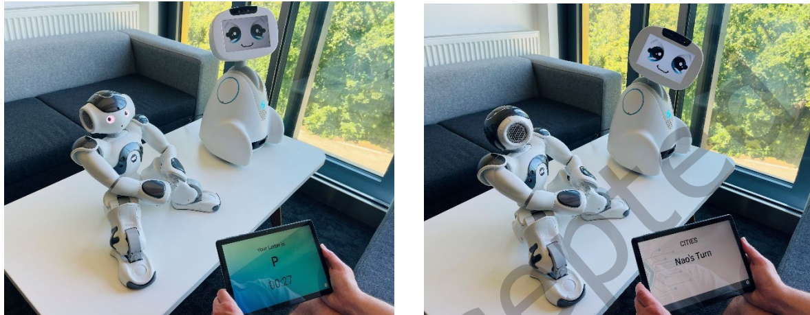
Figure 1: The setup of the multi-party game with the two robots (NAO: left, Buddy: right) and the human participant. The game is self-directed by the participant through the tablet-based application, the interaction occurs autonomously and in natural language between the involved parties. The robots simulate a "natural" behaviour, for example, by turning heads when talking to each other and then facing back the participant, or performing animated gestures.
