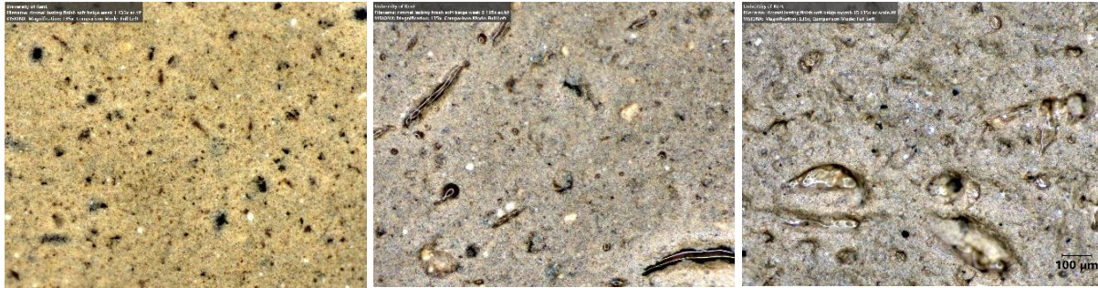
Figure 5.20: Colour photomicrograph images of Rimmel Lasting Finish Foundation (x135 magnification), taken from the sample placed on a glass microscope slide and allowed to age in air and natural light, (L-R) week 1 (freshly opened), week 5, month 15.
