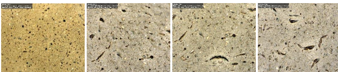
Figure 5.13: Colour photomicrograph images of Rimmel Lasting Finish Foundation (x75 magnification), taken at weekly intervals, showing a marked decrease in fluid content over time, (L-R) week 1 (newly opened), week 2, week 3, week 4.
