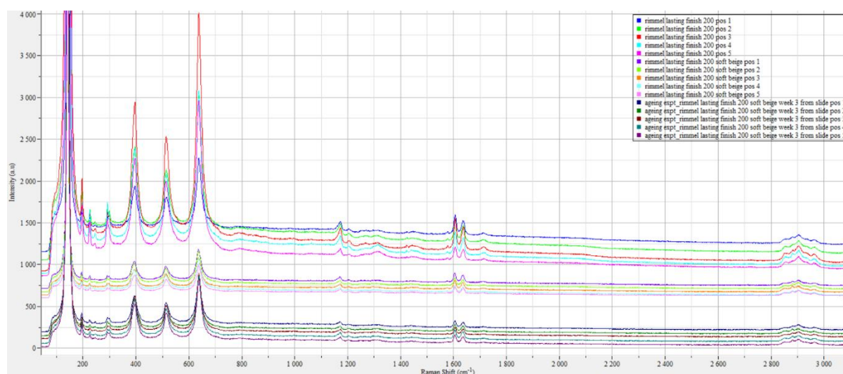
Figure 6.12: Raman spectra (unprocessed but stacked for clarity) of three Rimmel Lasting Finish Foundations in shade 200 Soft Beige: donated sample (top five spectra), new sample purchased in 2020 (middle five spectra), new sample purchased in 2023 (bottom five spectra).
