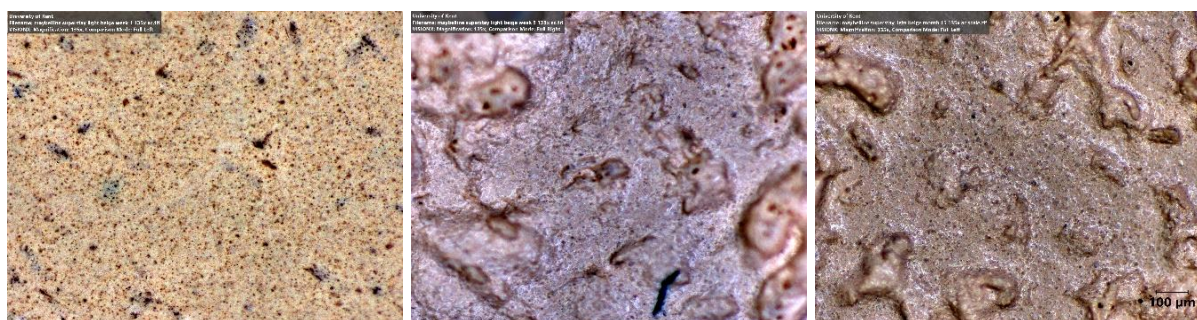
Figure 5.19: Colour photomicrograph images of Maybelline Superstay Foundation (x135 magnification), taken from the sample placed on a glass microscope slide and allowed to age in air and natural light, (L-R) week 1 (freshly opened), week 5, month 15.
