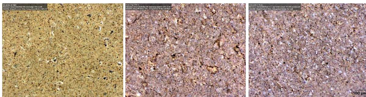
Figure 5.17: Colour photomicrograph images of L'Oreal Infallible Foundation (x135 magnification), taken from the sample placed on a glass microscope slide and allowed to age in air and natural light, (L-R) week 1 (freshly opened), week 5, month 15.
