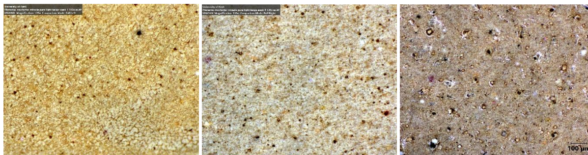
Figure 5.18: Colour photomicrograph images of Max Factor Miracle Pure Foundation (x135 magnification), taken from the sample placed on a glass microscope slide and allowed to age in air and natural light, (L-R) week 1 (freshly opened), week 5, month 15.
