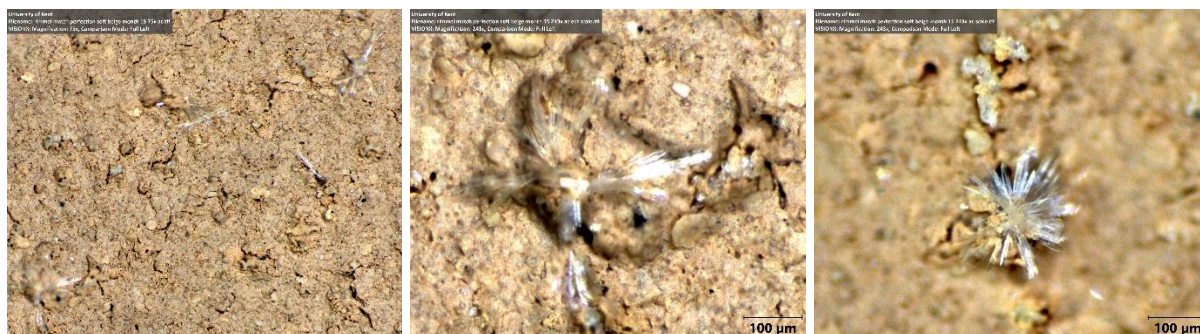
Figure 5.22: Colour photomicrograph images of Rimmel Match Perfection Foundation taken from the sample placed on a glass microscope slide and allowed to age in air and natural light for 15 months, (left) image at x75 magnification showing several fibrous mineral structures, (centre) one of the mineral structures taken at x243 magnification, (right) two different mineral structures taken at x243 magnification.
