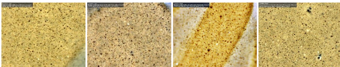
Figure 5.2: Colour photomicrograph images of Bourjois Healthy Mix Foundation (x135 magnification), taken directly from the bottle at various time intervals after product opening, (L-R) week 1 (newly opened), week 5, week 9, month 15.
