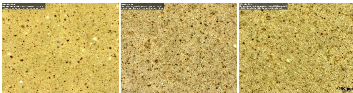
Figure 5.15: Colour photomicrograph images of BareMinerals BarePro Foundation (x135 magnification), taken from the sample placed on a glass microscope slide and allowed to age in air and natural light, (L-R) week 1 (freshly opened), week 5, month 15.
