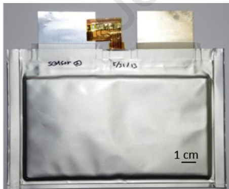
(a) Thin Film thermocouples embedded inside Li pouch cells [67].
