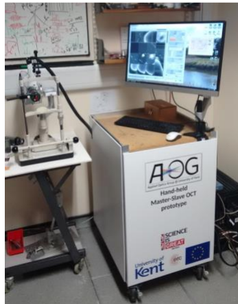
Fig. 4. OCT multifunctional system on a trolley
