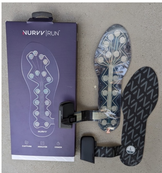
Figure 16: Photo of insoles (back and front) and packaging. The 16 sensors are clearly visible on the back of the insole.
