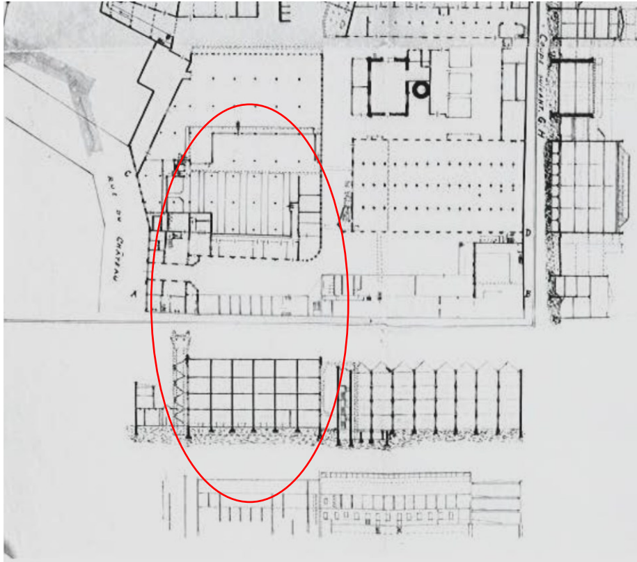
Figure 1.21: Plan, section and elevation of the Charles Six factory site, Tourcoing (architect unknown, 1897) in the 1980s with outline (circled) of the original wool-combing mill, undated. (M4178309. Archives Départementales du Nord)
