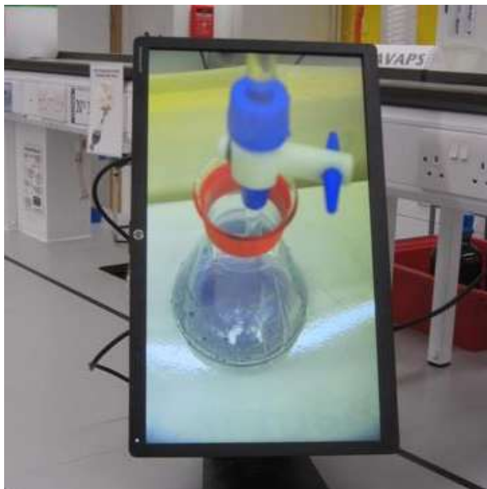
Figure 10 Webcam display. Image of the titre flask captured by a webcam and displayed on a screen allowing the student to observe the endpoint of the reaction without needing to get close to the flask and chemicals.
