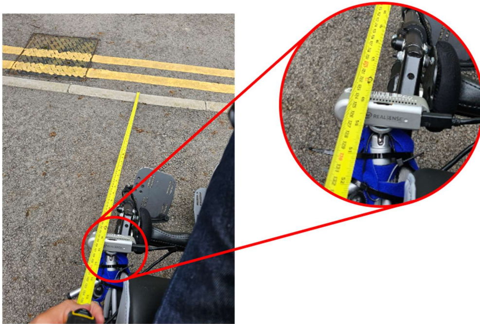
Figure 6.22: PEARS2 Traversable Area. The traversable area ground truth as measured by the tape measure. The distance is 1.23 meters.
