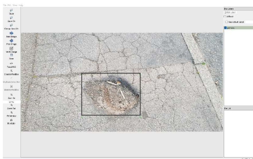
Figure 3.4: Image labelling as completed using the open-source software described in this section. In the image, the pothole object has been surrounded by a manually-drawn bounding box labelled as “pothole”. This will serve as an indication to the object detector during the training process.
