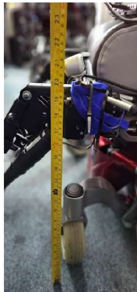
Figure 5.8: Experiment setup. Intel RealSense D435i fitted at 53 cm from the ground.
