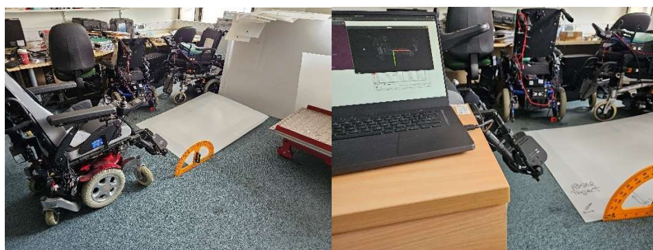
Figure 5.9: Isolated environment experiment. The wheelchair was parked in front of a manually built inclined platform with variable inclinations measured by a protractor in order to provide the ground truth information.
