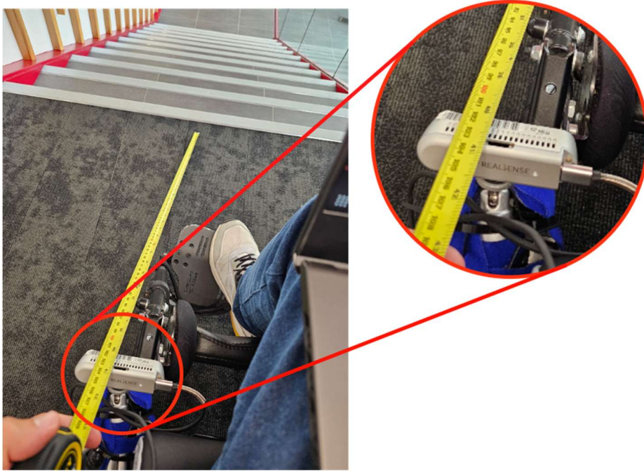
Figure 6.17: KENEDYST1 - Distance Centre . The ground truth for the distance from the camera sensor to the centroid of the segmented plane observed via the algorithm as measured by the tape measure. The measured distance is 1.02 meters.
