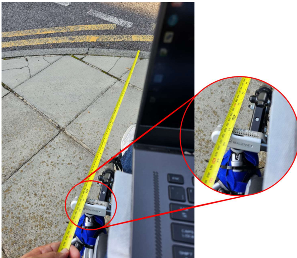
Figure 6.14: GRIMOND2 Traversable Area . The traversable area ground truth as measured by the tape measure. The distance is 1.54 meters.
