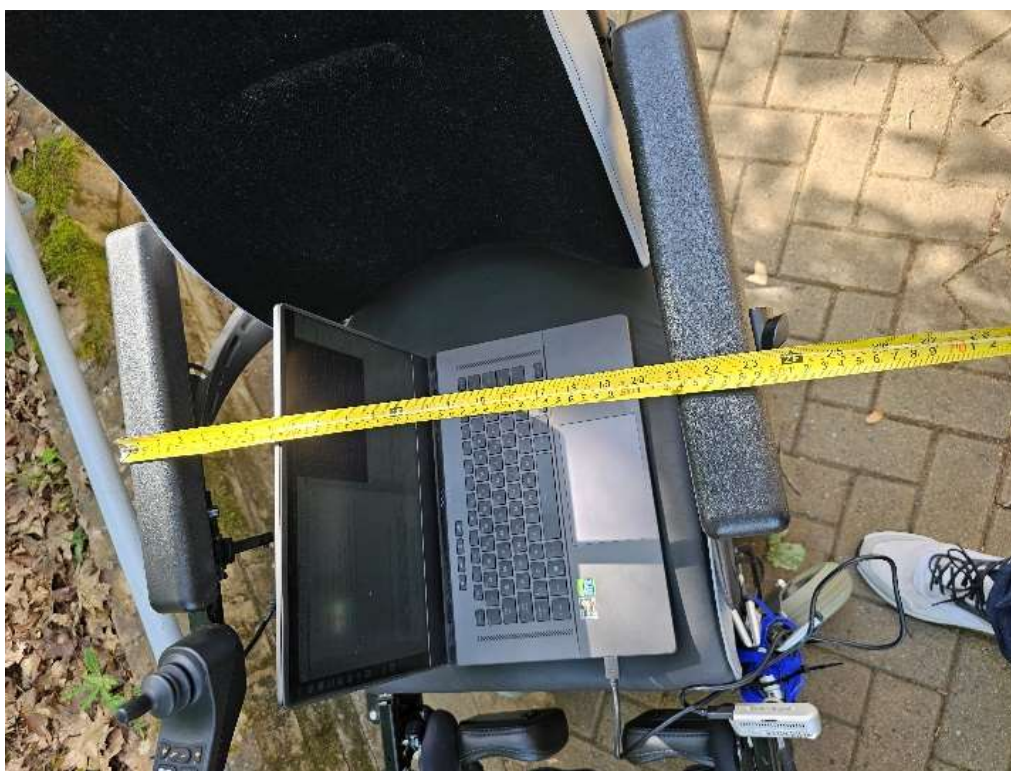
Figure 5.2: Width of the Electric-Powered Wheelchair.
