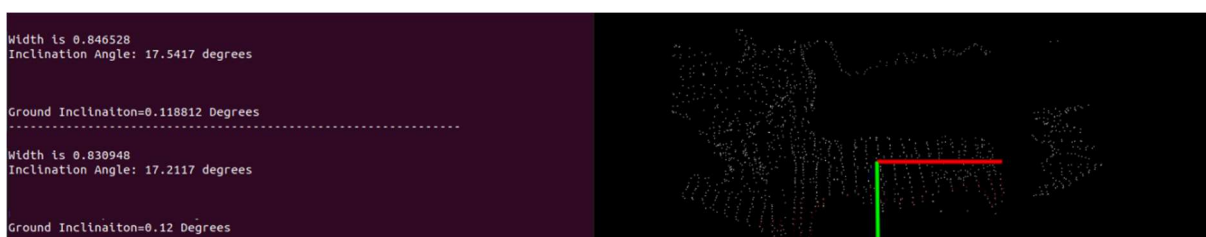
Figure 5.21: "Lab 16" Instance experiment result as returned by the proposed algorithm. The figure represents the segmented plane (right) and the returned results (left). The estimated inclination as measured by the algorithm is more than 17 degrees, and the angle width is less than 1 meter, hence the ramp being considered as not traversable.
