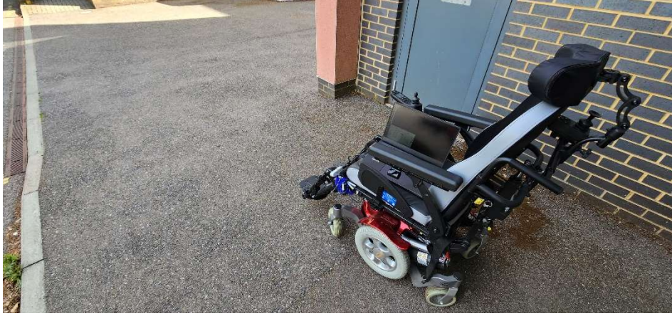
Figure 6.5: Experiment setup. The Salsa M2 Electric-Powered Wheelchair with the D435i mounted onto the left footrest upper hinge.
