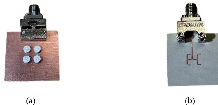
Figure 13. Photographs of the FDM 3D-printed DRA array with an in-phase feeding network. (a) top view, (b) bottom view.
