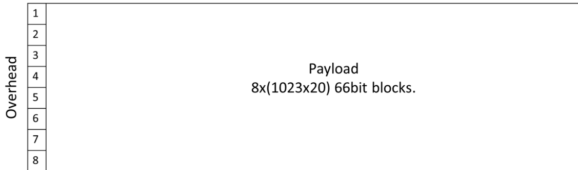
Fig. 2.14: FlexE multi-frame structure [19].
