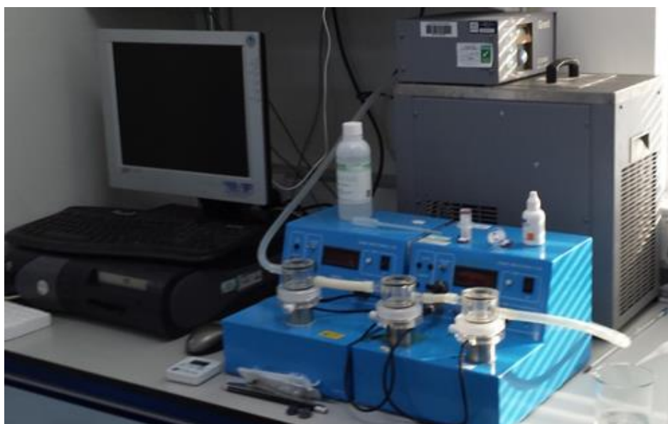
Figure 2.2. Oxygen Electrode Apparatus. The oxygen electrode (blue) consists of chambers that are connected to temperature-controlled circulating water bath.
