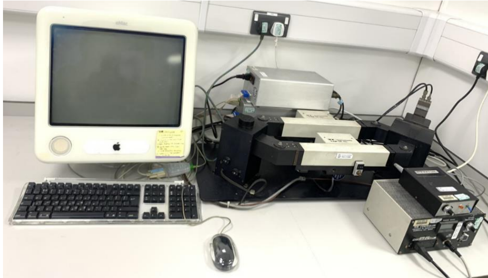
Figure 2.1. SDB4 Spectrophotometer. This is a special type of spectrophotometer that can analyse highly turbid samples.
