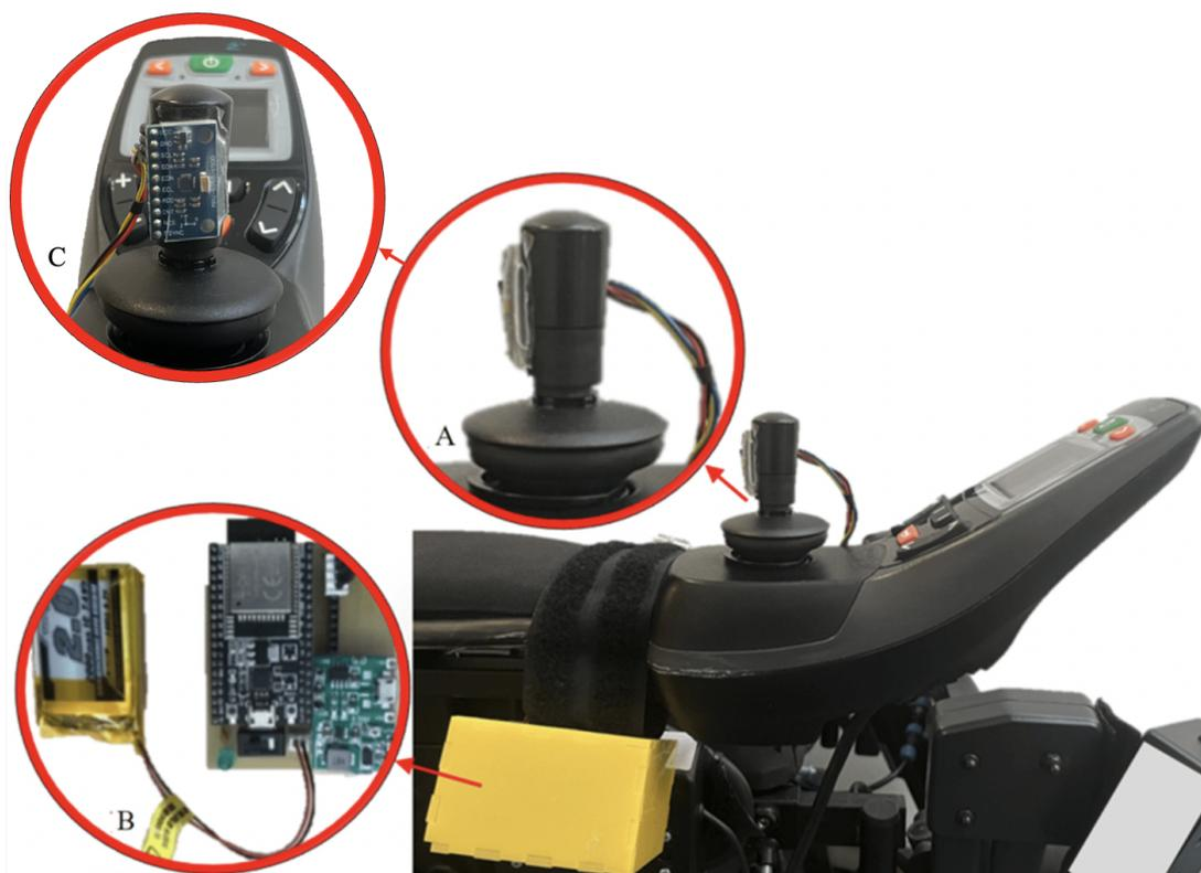
FIGURE 4.3: MPU-9250 sensor attached to the wheelchair's joystick (Dx2-REM550/551) to control the VR System. Inset A shows the MPU-9250 sensor on the joystick. Inset B shows the ESP-32 microcontroller and the battery that powers it (housed in the yellow case), which is wired to the MPU-9250 sensor and wirelessly sends signals to the Microsoft PC. Inset C shows the MPU-9250 sensor on the joystick from the front view.
