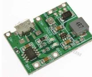
FIGURE 4.7: LiPo battery charger used to recharge the lithium-ion battery.
