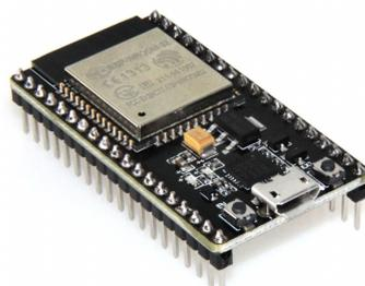
FIGURE 4.5: Microcontroller utilised for the controller: ESP-32.
