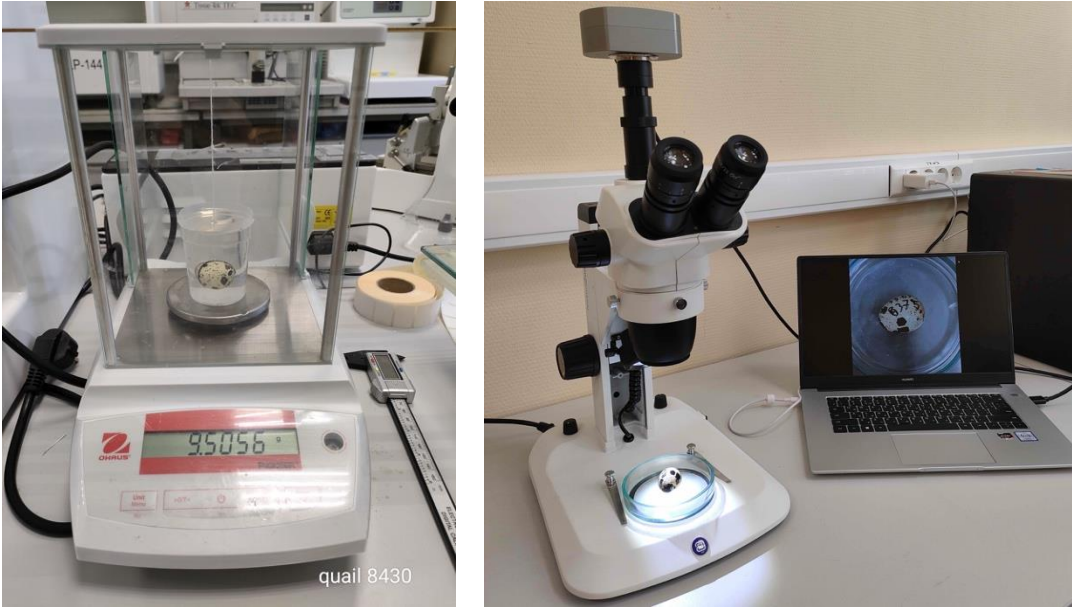
Fig. 1. Experimental setting for quail egg examination. (A) Hydrostatic weighing (a digital caliper gauge is also shown next to the digital scale). (B) Digital photographing.
