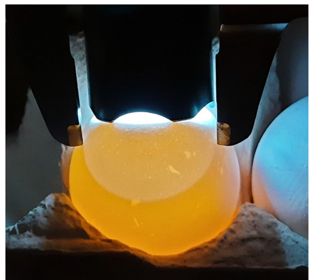
Fig. 1 The process of measuring the air cell diameter of an egg
