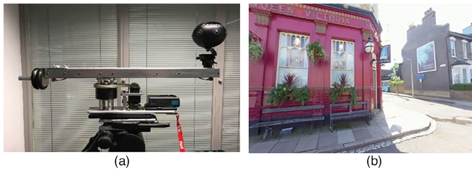
FIGURE 16 Background reconstruction using LF technology for production, (a) 360° motorised camera rig for LF acquisition, and (b) reconstructed background using Unity game engine [86, 87].
