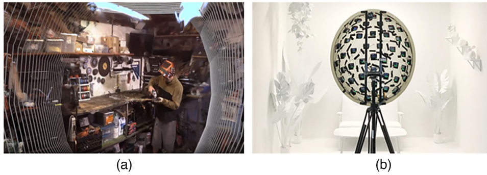
FIGURE 15 A system of acquiring and rendering LF video, (a) multi-sphere images, and (b) capture rig [15].
