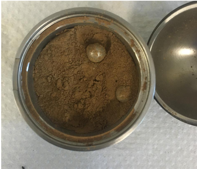
Figure 141. Photograph taken of the JSC-Martian simulant milled for 10 minutes at a frequency of 30 Hz utilising the Fritsch P23 mini mixer mill.
