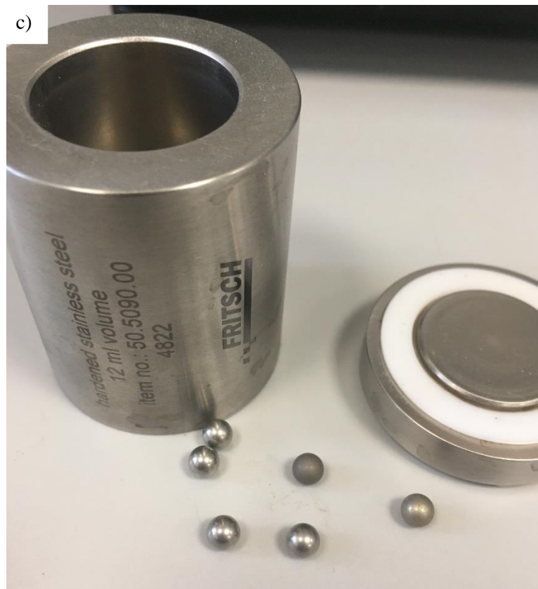
Figure 17. Photographs taken of empty stainless steel reaction vessels and ball bearings for a) Retsch MM301 mixer mill; b) Fritsch P23 mini mixer mill; c) Fritsch P7 planetary micromill.
