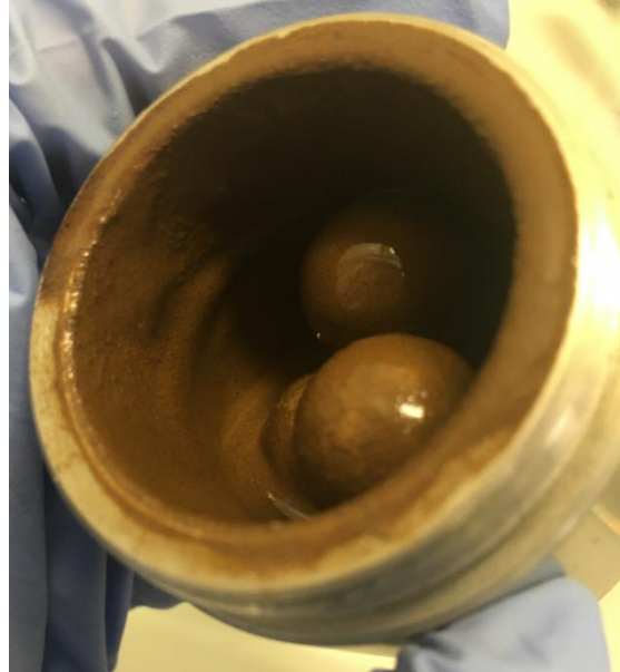
Figure 138. Photograph taken of the synthesised MGS-1 simulant milled (Retsch MM301 at a frequency of 10 Hz) with 25 % tap H 2 O ice for 10 minutes.
