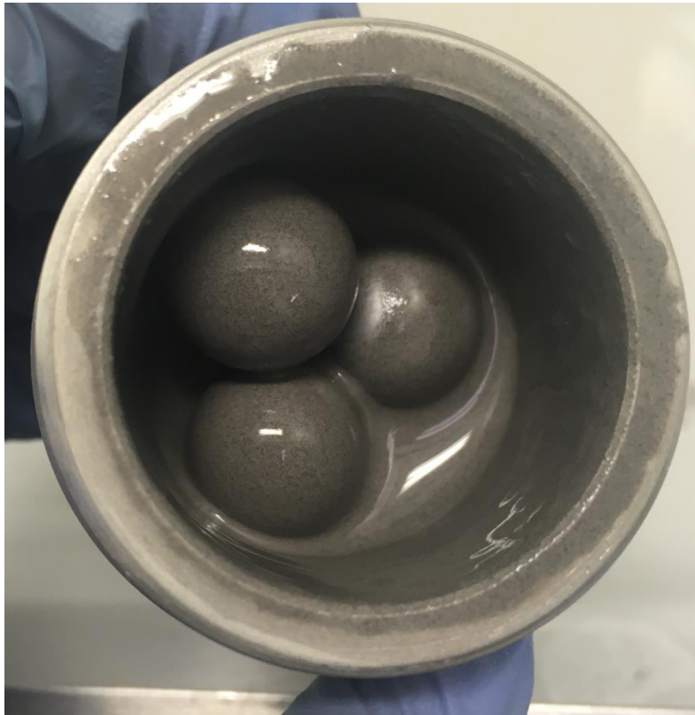
Figure 20. Photograph taken of LHS-1 simulant milled with 25 % deionised water ice after milling for 10 minutes using the Retsch MM301 mixer mill.
