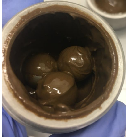
Figure 132. Photograph taken of the Earth-based JSC-Martian simulant milled (Retsch MM301 at a frequency of 10 Hz) with 25 % tap H 2 O ice for 10 minutes.
