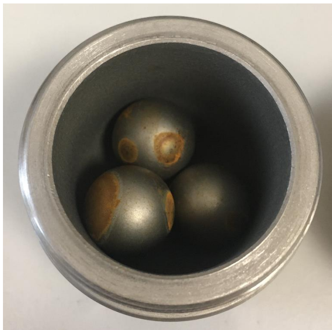
Figure 140. Photograph taken of 5 mm stainless steel ball bearings with iron rust residue.
