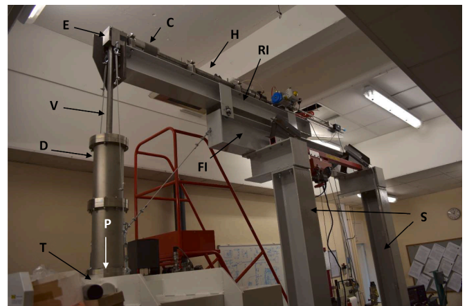
Fig. 1. Photograph of the new gun assembly. The horizontal first (pump) stage (H) is at the top of the image and the vertical second stage (V) (launch tube) assembly at the left. The central breech (C) is on the left-hand end of the horizontal pump tube. The right angle elbow then follows (E) connecting to the vertical launch tube. The larger internal diameter drift tube (D) physically connects the launch tube and the target chamber (T). The direction of the projectile as it enters the target chamber is indicated (P). The whole gun assembly is supported on two vertical steel columns (S), topped with a horizontal “I” beam fixed permanently in position (FI). The pump-tube and breech are mounted on a horizontal, rolling “I” beam (RI), which is in turn mounted on FI.
